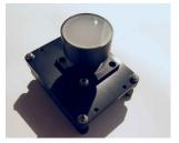
affords a clear un-obscured view of the sky. It is attached to the  $\mu$ -MCA by means of an electrical umbilical cable that is plugged into to a circular connector at the rear of the  $\mu$ -MCA. The umbilical carries power, ground and a serial trigger signal between the e-ILS and the  $\mu$ -MCA system. Extension cables are available for mounting the e-ILS up to seven meters away from the  $\mu$ -MCA system.
