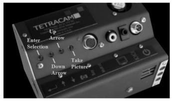
Navigation begins when the enter key is pressed. The first screen shows icons for the setup screens that are available to the user. The icons start small (1/2 size) and get larger when one of them is selected with up and down arrow keys. In the illustration below, the tools setup icon has been chosen. This screen is used to delete images and format memory cards. These settings are preserved through power cycles. Pressing enter activates the tools screen.
