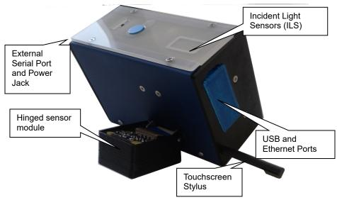
A stylus is stored at the corner of case. The stylus can be used to make touchscreen operation easier. An Ethernet connector allows the camera to be attached to a Local Area Network for unloading images and managing options
