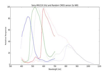
same for each of the red, green and blue bands when there is no blocking filter. The NIR response shown is empirically derived, and should not be used for precise calculations.
