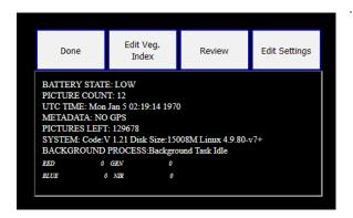
The status information is updated once per second. Battery state is shown, along with image counts and storage use. ILS measurements are shown in live bars at the bottom of the info screen.
