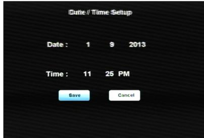
The clock settings are standard except for the UTC offset field. Here the user enters the difference in hours between local time and UTC (Greenwich, U.K.). The default UTC value is pacific daylight time (Chatsworth, CA), or -8.
