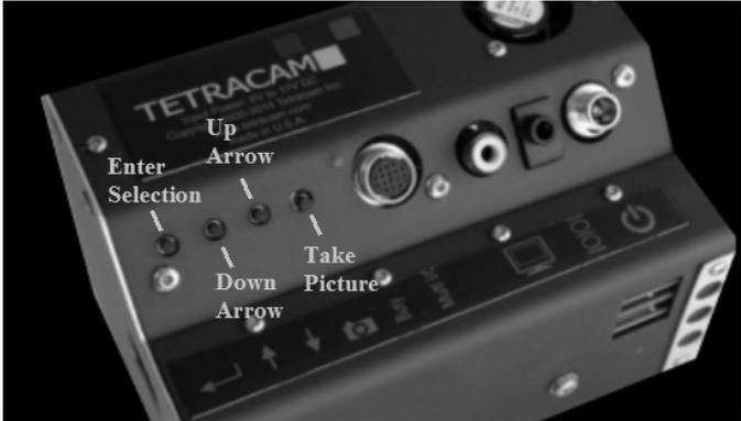
Navigation begins when the enter key is pressed. The first screen shows icons for the setup screens that are available to the user. The icons start small (1/2 size) and get larger when one of them is selected with up and down arrow keys. In the illustration below, the tools setup icon has been chosen. This screen is used to delete images and format memory cards. These settings are preserved through power cycles. Pressing enter activates the tools screen.
