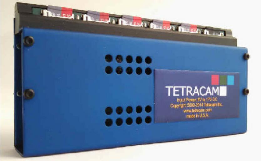
When the Six Pack is populated with a set of cards from a mission, it looks exactly like the camera array to PixelWrench2, and all camera processing operations can proceed as if the host computer were connected to a  $\mu$ -MCA.
