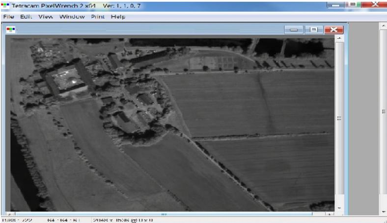
PixelWrench2 oversees transfer of images from the  $\mu$ -MCA system's image memories to the host computer. It provides tools for managing  $\mu$ -MCA image sets, complex batch processing tools, extraction of several vegetation index and canopy segmentation images as well as a comprehensive suite of image editing tools. PixelWrench2 translates Tetracam's proprietary DCM10, RAW10 and RAW8 image files into standard image file types (BMP, JPEG, TIFF, PNG etc.)
