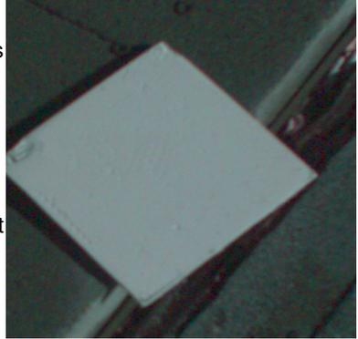
Place the calibration target on the ground, or hold it level with the ground, and photograph it. It need not fill the entire frame and it must not be overexposed. Make sure to avoid a direct reflection of the sun. The sample image on the left is of a properly exposed calibration target. When the pictures are imported to the host computer, the calibration image will be used to refine the vegetation index calculations.
