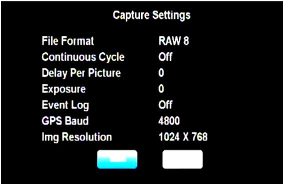
File Format selects if picture data will be compressed, or saved as it comes out of the sensor (RAW) for speed.
