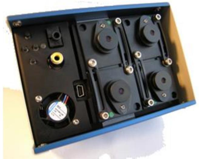
Important in vegetation analyses. All cameras in the array are registered and synchronized so that each captures the same image at the same time at a different band.
