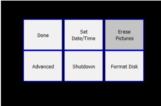
The tools page provides buttons for managing the state of the camera. Images can be erased, the image storage partition can be formatted, and the camera can be shut down. The page also has an ADVANCED button that allows the camera settings to be
