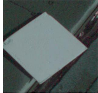
Place the calibration target on the ground, or hold it level with the ground, and photograph it. It need not fill the entire frame and it must not be overexposed. Make sure to avoid a direct reflection of the sun. The sample image above is of a properly exposed calibration target. When the pictures are imported to the host computer, the calibration image will be used to refine the vegetation index calculations.
