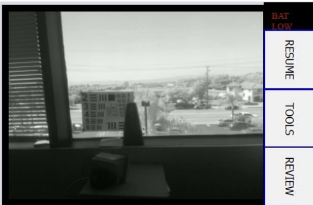
After each picture is captured using the picture taking button, the screen will freeze, showing the frame captured. Tapping RESUME re-establishes the live view.
