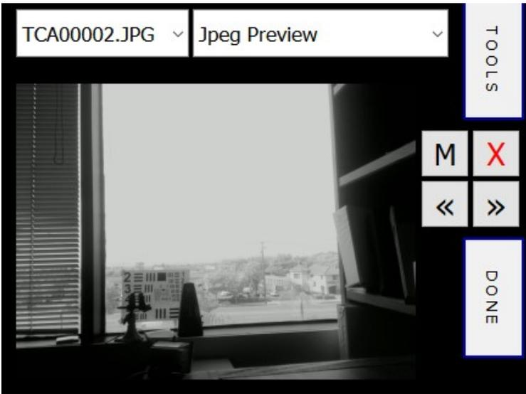
The Jpeg Preview image has been optimized for touchscreen viewing, and does not always reflect the brightness and contrast of the raw data. To see the finished picture quality, an RGB extraction should be used. The RGB extraction shows the illumination and contrast of the final image correctly.
