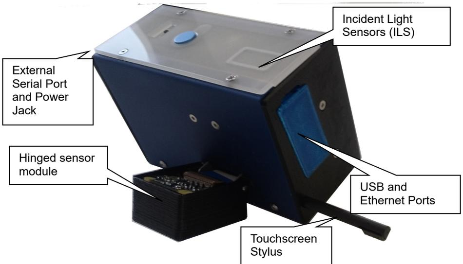
A stylus is stored at the corner of case. The stylus can be used to make touchscreen operation easier. An Ethernet connector allows the camera to be attached to a Local Area Network for unloading images and managing options
