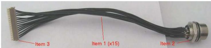
Item 3 in the above photo is the mating connector for the ADC Snap. The wires (Item 1) are about 3 inches in length, and carry the connections to the round Hirose Bulkhead connector, Item 2. The pins on the ADC Snap connector map to the Hirose connector as shown in the following diagram:
